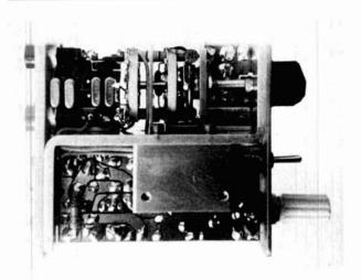
Converter bottom view. At upper right is the printed circuit supporting the rf trimmers, followed by the bandswitch and, at the left, the crystals (the 13-MHz crystal is missing). Below the central aluminum element is the lower part of the main printed circuit together with its supporting bracket.
